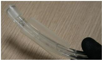
Next, pushing the connector pin into the start of the rope light length.
