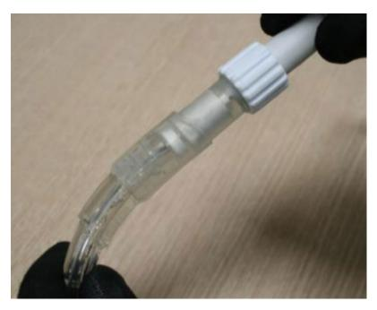
Repeat this on the end of the rope light, to seal the end cap in place
